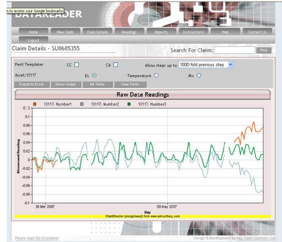
DataREADER interprets data from the new range of sensors using telemetry. This application retrieves data from the suppliers web site, graphs it and interprets it plus produces a report with just a few keystrokes by the user.
